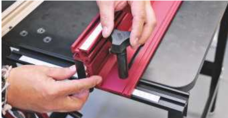
▲ The fence locks into 'T' slots on the side extrusions and runs slickly
